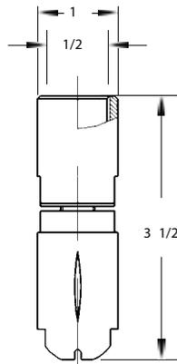
UBF type rotary tank washer nozzles contain all the features of the UBC series, but are designed to operate in smaller size tanks that contain relatively limited size openings such as found in pressurized soft-drink containers and beer kegs.
