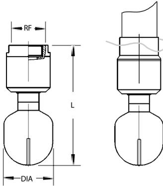
UBC type rotary tank washer nozzles contain slotted, flat-shaped spray orifices positioned such that the jets provide the reaction forces to produce the rotary motion. This simple yet robust design, utilizing two ball bearing assemblies, makes it possible to operate the nozzle in any orientation, giving an efficient 360° of coverage.
